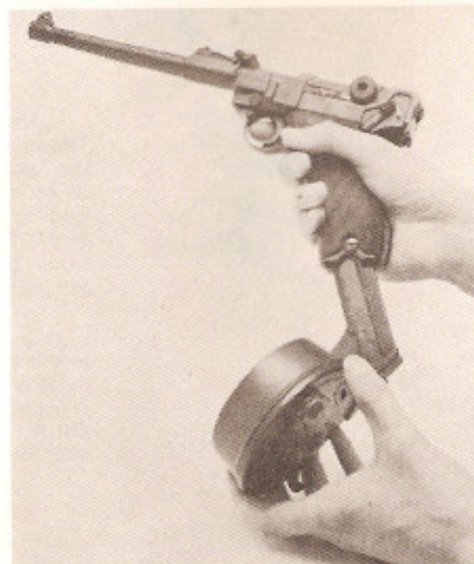
A replica 32-round Snail Drum magazine is available as an accessory for the "Artillery" Model pistol
